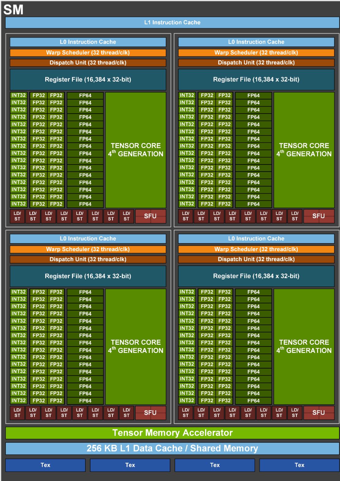
Figure 7. GH100 Streaming Multiprocessor (SM)
